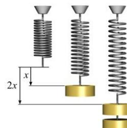
If we pull a spring it gets longer when we exert more force to it. We can see that when we apply double the force on the spring, it gets twice as long. Therefore, the extension of the spring ( $x$ ) is **directly proportional to the force applied to it ( $F$ )**. This is the conclusion drawn by the English physicist **Robert Hooke** in 1660 and that is why it is called **Hooke's Law**:
