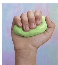
We can find many solid objects all around us. If we push or pull an object, it may be deformed (change its shape) permanently, like plasticine or modelling clay (**plastic materials**) or not, like a spring or a hairband (**elastic materials**).
